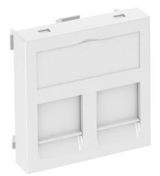
Data technology support with straight outlet and locking slider to accept two data technology connection modules with RJ45 socket. The locking fastening is suitable for horizontal and vertical installation in the system environment. Type PA has a special module seat and is designed for indirect fastening of the data connecti-
