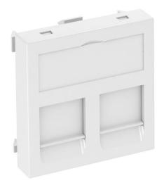
Data technology support with straight outlet and locking slider to accept two data technology connection modules with RJ45 socket. The locking fastening is suitable for horizontal and vertical installation in the system environment. Type A has a mounting opening of 20.10 x 14.80 mm and is designed for direct fastening of the data connection modules in the mounting opening.
