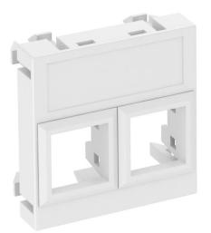
Data technology support with straight outlet and without a locking slider to accept two data technology connection modules with RJ45 socket. The locking fastening is suitable for horizontal and vertical installation in the system environment. Type LE has a special module seat and is designed for indirect fastening of the data connection modules in the mounting opening.
