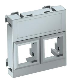
Data technology support with straight outlet and without a locking slider to accept two data technology connection modules with RJ45 socket. The locking fastening is suitable for horizontal and vertical installation in the system environment. Type LE has a special module seat and is designed for indirect fastening of the data connection modules in the mounting opening.
