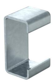
Spacer for use in US 5 support or in the head plate, type KU 7 VQP. For static reasons, the spacer is always used to increase stability to prevent the support from deforming when the bracket is tightened with the hexagonal bolts.
