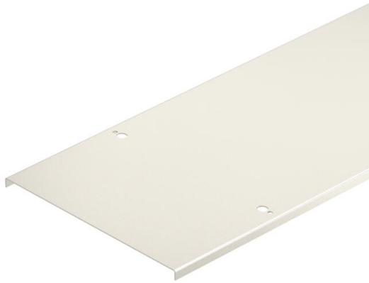
Lid for stand-off mounting. Not suitable for the vertical ladders SLM and SLS. Spacers must be ordered separately for every 3 m under article number 6065475 for cable trays and cable ladders as well as under article number 6065477 for wide span systems. When using covers outdoors, additional measures against the influence of wind must be taken.
