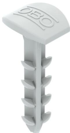
Push-fit plug Delta-Push® for mounting electrical installations. Suitable for concrete, calcareous limestone, full brick, hollow brick and porous concrete. Toolless mounting by pushing into a drill hole in a wall or on a ceiling. Without screws. To install cable trunking or labelling panels, for example.
