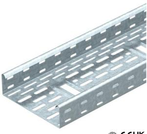
DKS 60 = perforated cable tray system with 60 mm side height. Permeable cable tray system to VdS guideline 2092 with 30% hole surface for use under sprinkler systems. Bottom penetration from width 200 mm.
