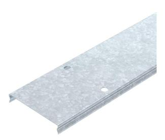
Lockable cover for mesh cable trays of type GR and GRM. Protects cables from damage, contamination and moisture from above. Suitable for industrial areas such as mechanical engineering. With transverse bead from 400 mm width.
