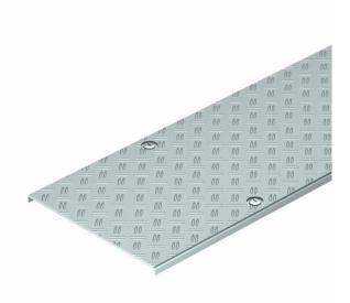
Cable tray cover for the walkable BKRS cable tray system. The basic cover is strip galvanised in a material thickness of 2 mm with additional aluminium chequer riveted on in a thickness of 4 mm, sturdy and non-slip. Turn buckle fastening with a turn buckle distance of 500 mm.
