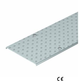
Cable tray cover for the walkable BKRS cable tray system. The basic cover is strip galvanised in a material thickness of 2 mm with additional aluminium chequer riveted on in a thickness of 4 mm, sturdy and non-slip. Turn buckle fastening with a turn buckle distance of 500 mm.
