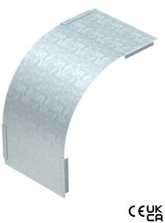
Cover for falling vertical bends of side height 60 mm. The fastening is guaranteed by the overlap of the cable tray covers. The cover can also be fastened using cover clamps.
