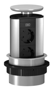
Lowerable Deskbox with connection cable for fixed installation on a tabletop, plastic fastening sleeve, painted accordingly in cover shade. It is mounted using a drill hole (Ø102 mm) in the tabletop.
