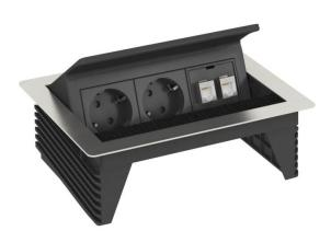
Foldable Deskbox with connection cable for fixed installation in a tabletop, housing made of brushed stainless steel with brush bar as cable outlet. Mounting is done via an installation opening 195 x 157 mm in the tabletop.
