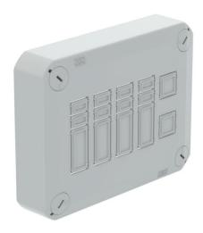
Pluggable cover for the closing of junction boxes, equipped with 6 break-out openings for connection sockets by Wieland and Wago, 3- to 5-pole. With quick lock in cover, sealable. Halogen-free material, UV-resistant Flame-resistant to DIN EN 60695/2/11, test temperature 650 °C. Impact resistance IK07 at room temperature. Protection class IP30.
