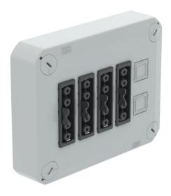
Pluggable cover for the closing of junction boxes, equipped with 4 Wieland GST18 plug systems, prewired with lever plug-in connectors. With quick lock in cover, sealable. Halogen-free material, UV-resistant Flame-resistant to DIN EN 60695/2/11, test temperature 650 °C. Impact resistance IK07 at room temperature. Protection rating IP30
