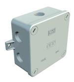
B 9 K ...: Protection IP67 Empty box to be used with single terminals 4 cover screws of plastic, so fully corrosion-proof 2 fixing holes for screws up to 5 mm diameter 7 breakout entries with Pg 16 thread, with 3 cable glands of polyamide for cable diameters of 10–14 mm type 106/16 B9K The cable glands have a specially shaped thread which automatically breaks out the entry when the gland is screwed in.
