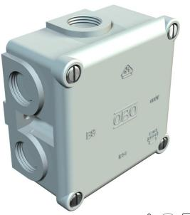
Protection rating IP54, nominal voltage 660 V, nominal cross-section 2.5  $\div$  mm<sup>2</sup>, two fastening holes for screws up to 5 mm Ø on the outside of the box, four cover screws, 7 break-out entries with thread M20 x 1.5, primarily for cable glands with short connecting thread.
