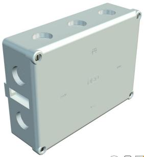
Protection rating IP54, nominal voltage 660 V, nominal cross-section 16  $\div\,$  mm², two fastening holes for screws up to 6 mm Ø on the outside of the box. Four cover screws, 10 break-out entries with thread M25 x 1.5.
