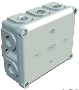
Protection rating IP54, nominal voltage 660 V, nominal cross-section  $10 \div mm^2$ , two fastening holes for screws up to 6 mm Ø on the outside of the box, four cover screws, 10 break-out entries with thread M20 x 1.5, primarily for cable glands with short connecting thread.
