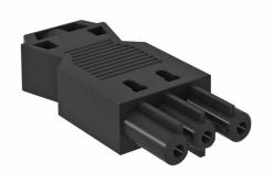
Socket part, 3-pin, type GST18i with screw connection, low height (no slot loss in combination with distributor blocks), for cross-sections of 0.75–2.5 mm², single-and fine-wire cables connectable without end sleeve, for cable diameters between 6.5–10.5 mm (H05VV, NYM), unmounted with strain relief, terminable in situ, 250 V, 16 A.
