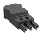
Socket section, 3-pin, type GST18i with screw connection for cables of 1.5–4.0  $\,$  mm² and for cable diameters between 10.5–14.5 mm (H05VV, NYM), unmounted with strain relief, terminable in situ, 250 V, 16 A.
