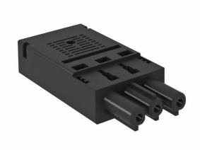
Socket part, 3-pin, type GST18i with spring power connection for rigid cables of 1.5–2.5 mm², single-wire and ultrasonically welded, fine wire cables 1.5 mm² with end sleeves, unmounted with strain relief, can be terminated in situ, 250 V, 16 A.
