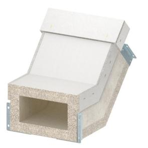
Rising vertical bend for PYROLINE® Con S fire protection duct, type BSKH09-K1021, consisting of fibreglass lightweight concrete which is resistant to water and frost for the creation of vertical changes of direction (45°) of the duct. Mounted connectors ensure quick mounting in situ, whilst loosely placed covers ensure quick inspection and reassignment.
