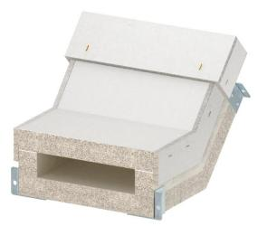
Rising vertical bend for PYROLINE® Con S fire protection duct, type BSKH09-K0521, consisting of fibreglass lightweight concrete which is resistant to water and frost for the creation of vertical changes of direction (45°) of the duct. Mounted connectors ensure quick mounting in situ, whilst loosely placed covers ensure quick inspection and reassignment.
