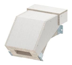
Falling vertical bend for PYROLINE® Con S fire protection duct, type BSKH09-K0511, consisting of fibreglass lightweight concrete which is resistant to water and frost for the creation of vertical changes of direction (45°) of the duct. Mounted connectors ensure quick mounting in situ, whilst loosely placed covers ensure quick inspection and reassignment.
