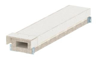
Fire protection duct made from water and frost-proof fibreglass light concrete of building material class A1 according to EN 13501-1 for fireproof laying of cables in rescue and emergency routes, and for the maintenance of electrical functionality of safety-relevant systems. Classification I90 as I duct according to DIN 4102 Part 11 and classification E30 as E duct according to DIN 4102 Part 12.
