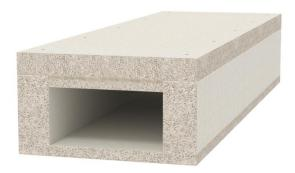
Fire protection duct made from water and frost-proof fibreglass light concrete of building material class A1 according to EN 13501-1 for fireproof laying of cables in rescue and emergency routes, and for the maintenance of electrical functionality of safety-relevant systems. Classification I120 as I duct according to DIN 4102 Part 11 and classification E90 as E duct according to DIN 4102 Part 12.
