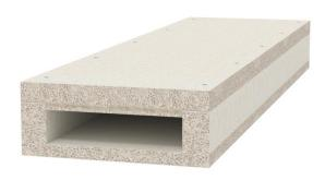
Fire protection duct made from water and frost-proof fibreglass lightweight concrete of building material class A1 according to EN 13501-1 for fireproof laying of cables in rescue and emergency routes, and for the maintenance of electrical functionality of safety-relevant systems. Classification I90 as I duct according to DIN 4102 Part 11 and classification E30 as E duct according to DIN 4102 Part 12
