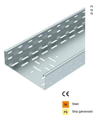
Perforated cable tray for the routing of cables, especially suited for material handling technology in the automotive industry. Can be used in indoor areas. Screw connection. Suitable for direct and elevated floor mounting.
