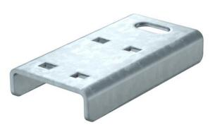
The connection component is the connection between the threaded rod lock and the suspension system for the routing types with cable trays for the maintenance of electrical function to DIN 4102 Part 12. Including bolts and nuts.
