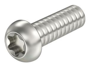
Flat head screw with TX 30, according to ISO 7380-1, suitable for fastening cable routes on brackets as well as for the mounting of barrier strips. The rounded head shape provides optimum cable protection. The Torx drive offers optimum force transmission in the screw movement.
