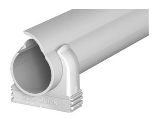
Set consisting of Quick pipe electrical installation pipes and Quick clip surface-mounted clips. For surface-mounted routing of cables in interiors and protected outdoor areas. Universal fastening on wall and ceiling. Comprises 40 m of pipe each of 2 metres in length and 120 Quick clips. Can be used in a temperature range of –25 to +60 °C.
