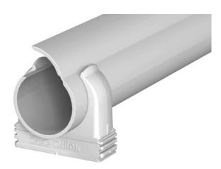
Set consisting of Quick pipe electrical installation pipes and Quick clip surface-mounted clips. For surface-mounted routing of cables in interiors and protected outdoor areas. Universal fastening on wall and ceiling. Comprises 50 m of pipe with each pipe 2 metres in length and 156 Quick clips. Can be used in a temperature range of -25 to +60 °C.
