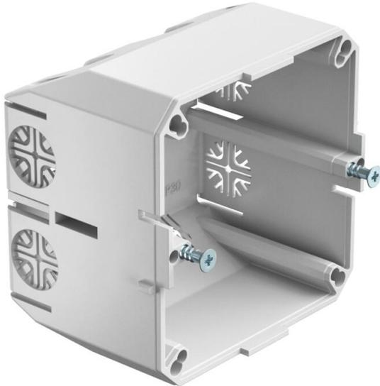
Accessory mounting box for the installation of devices with support rings and support clamps in WDK cable routing trunking of 60 mm trunking height. The device socket is placed on the floor connectors and fastened in the centre with a bolt.
