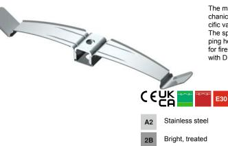
The metal pressure clip is halogen and fire load-free, and maintains a good mechanical stability even in fires. The pressure clip is also approved as a cable-specific variant for the maintenance of electrical functionality to DIN 4102 Part 12. The spacer 2033 D 15 x 3 G (must be ordered separately) increases the clamping height of pressure clips from 10 to 13 mm. The pressure clips are suitable for fireproof mounting above suspended fire protection ceilings in accordance with DIN 4102.
