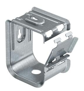
Metal grouped support for high mechanical stability, even in case of fire. Suitable for safe mounting above fire protection ceilings. Also approved as a cable-specific variant for the maintenance of electrical function to DIN 4102 Part 12. For wall and ceiling mounting. Lock can be opened without tools. Detailed information on the approved routing variants can be found in the appropriate testing documenta-
