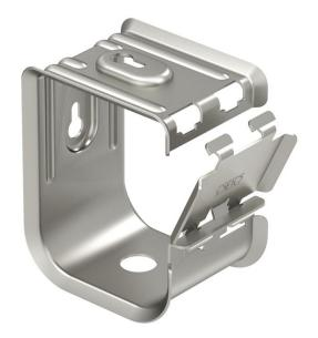
Metal cable tidy for high mechanical stability, even in case of fire. Suitable for safe mounting above fire protection ceilings. Also approved as a cable-specific variant for the maintenance of electrical functionality to DIN 4102 part 12. For wall and ceiling mounting. The lock can be opened without tools.
