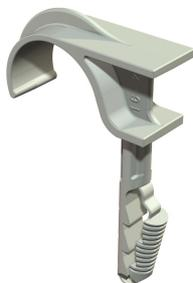
These push-fit clips are used when installing cables and pipes on walls and ceilings and when running flexible pipes on concrete and in the screed. The single push-fit clips can be used instead of nail clips in concrete and aerated concrete. The advantage of the push-fit clips is that they only have to be pushed into the drilled hole. Anchors and bolts are not needed.
