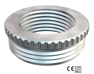
Reduction (Part H) to DIN 46320, with Pg thread to DIN 40430, as a transition from a PG thread hole to a smaller cable gland.
