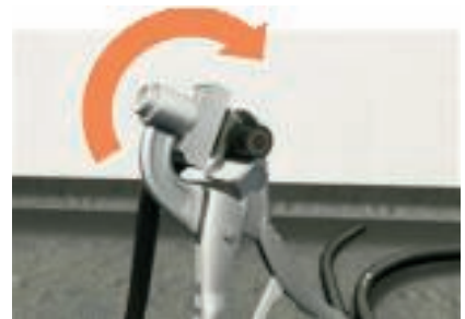
3. Apply the pliers and cut 25 mm of the jacketing, then turn it through 360°
