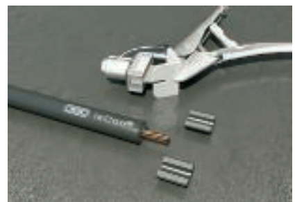
6. Turn the pliers to loosen the external jacket
