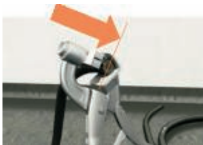
5. Cut the cable in a lengthwise direction on opposite sides
