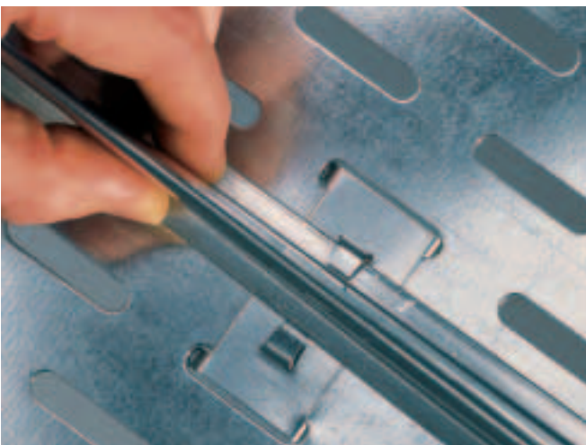
Inserting a TSG 60/S barrier strip: press together lightly and snap into place
