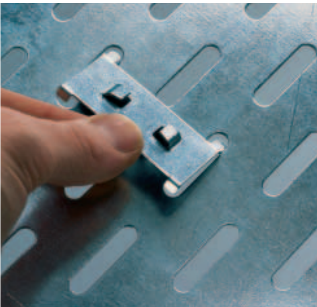
Inserting a KS MKS/SKS clamping bracket into an MKS cable tray (at intervals of approx. three units/stock length)
