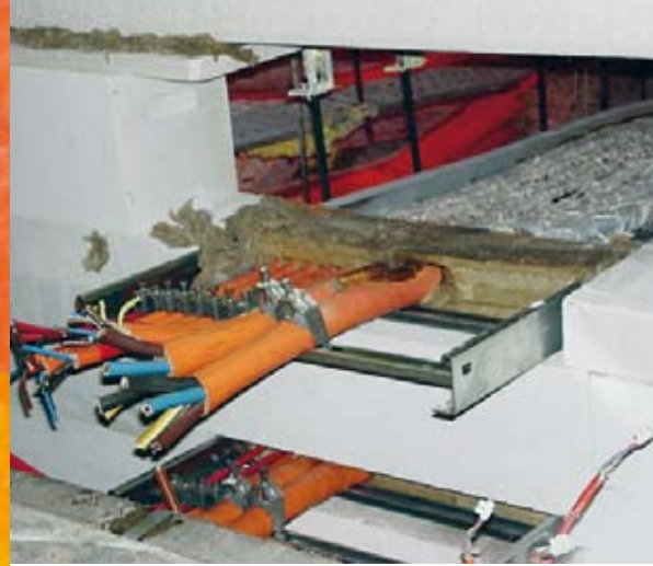
A glimpse into the testing furnace: glowing of the support structure, cable with insulating layer of ash
