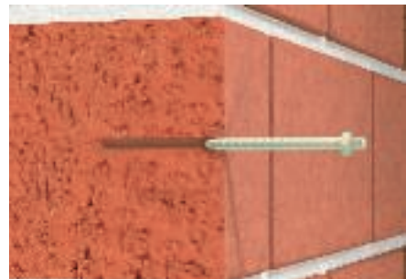
Fixing the fire protection bolt tie
