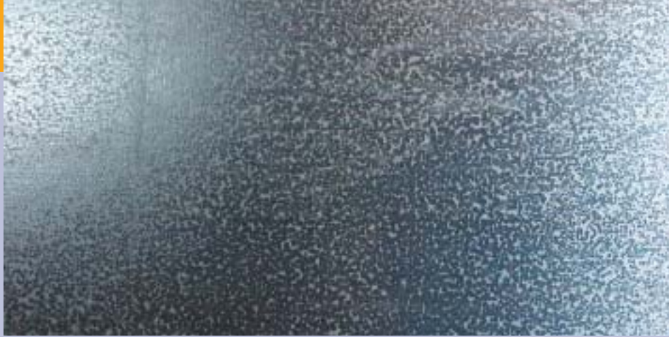
ball impact test: individually galvanised
