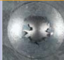
ball impact test: individually galvanised
